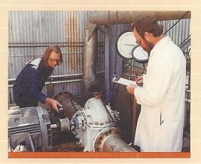
TEST LAB: Rigorous prototype testing is conducted to verify hydraulic performance, NPSH requirements as well as vibration and noise. These tests are conducted in strict accordance with Hydraulic Institute Standards. Ongoing production testing assures actual production units meet published performance. Instruments are calibrated and traceable to the U.S. Bureau of Standards.
