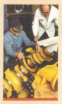
QUALITY CONTROL: Ongoing quality assurance/control is essential to maintain product reliability. Here, a Quality Control inspector measures a critical point of the pump volute. Hydrostatic tests are performed in accordance with Hydraulic Institute Standards.
