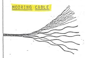
High flex 304 stainless steel. 7 x 19 x 3/16" (pictured) indicates cable consists of 7 bundles, each containing 19 strands, and has an outside diameter of 3/16". Larger size cables have greater outside diameters, 1/4" or 3/8", but still contain 7 bundles of 19 strands each.
